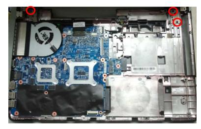
Loose screw of hinge to L-case, take off LCD module from L-case.
